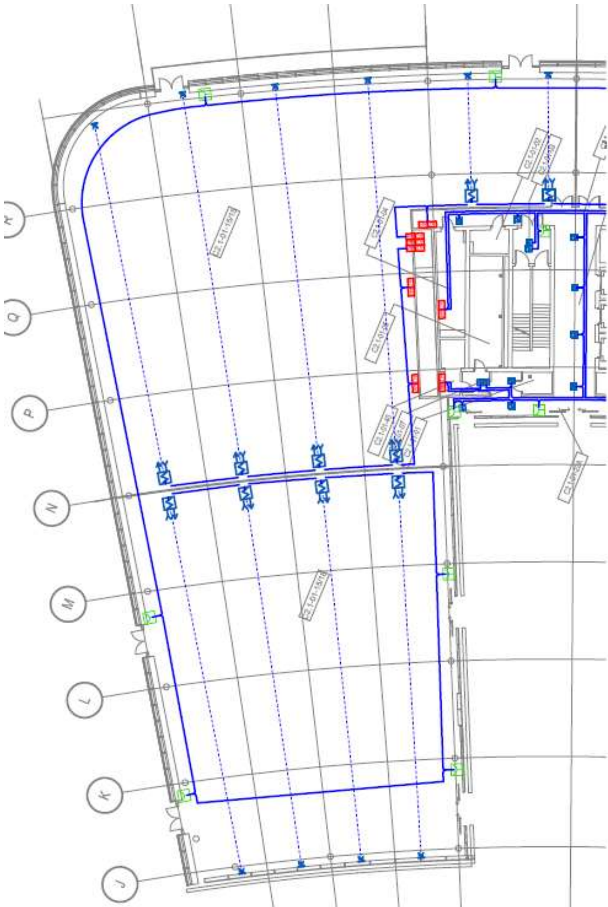
Figure 18: Rough plan of the automatic fire alarm detector layout in the Official Participant's Pavilion on the Facility 1st floor.
