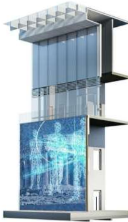
Figure 14. Fragment of internal façade (atrium) finishing H=9.8 m high.
