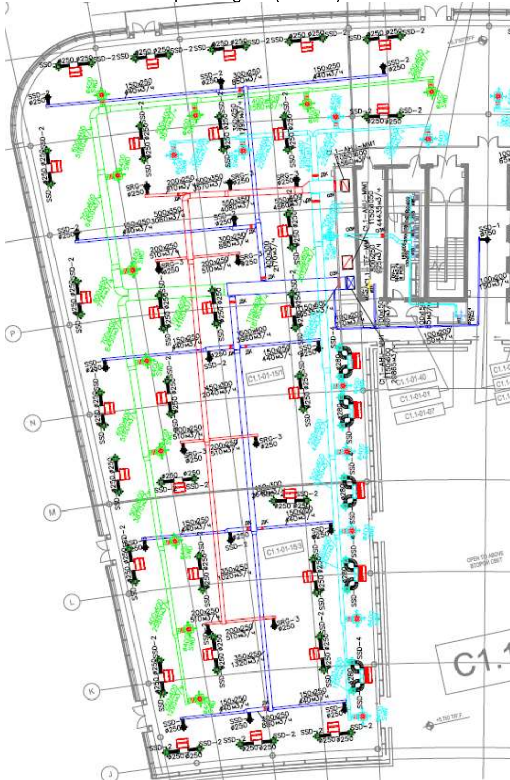
Figure 24: Rough layout of balanced ventilation channels in the Facility in the Official Participants' Pavilions.
