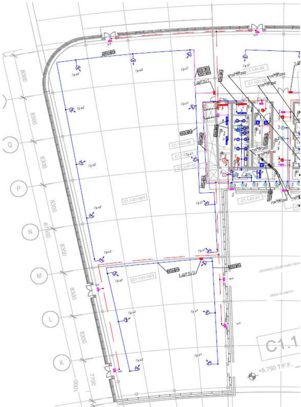
Figure 15: Official Participant switchboard (1-ShchR 15/3, 15/1) rough layout.
