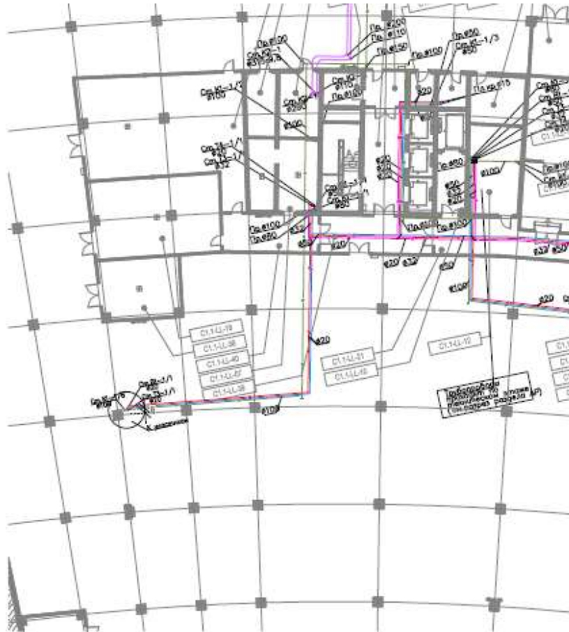
Figure 21: Plan showing location of waste water sewage supply to the Official Participant's Pavilion.
